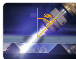
Bevel cutting with an angle of 50°
