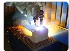
HotWire-cutting of non-conductive materials
