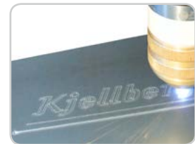
Marking with adaptable line width and depth
