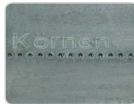
Punching with variable penetration
